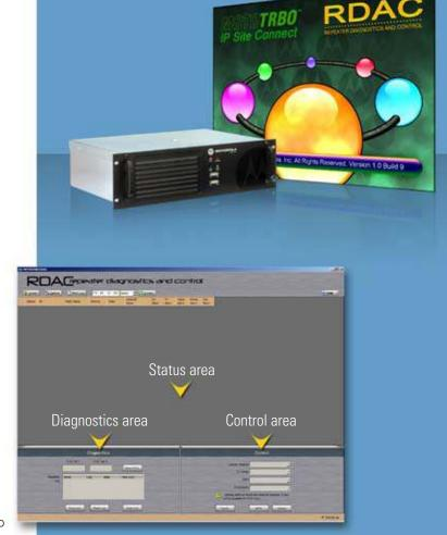
Can connect locally physically to one repeater, or connect via an IP network
