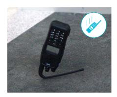
We drop them from 6 feet onto concrete – that's 50% higher than the MIL-STD-810G specification test. We drop each radio dozens of times from different angles, ensuring the durability of everything from battery and antenna fittings to internal components and the screen. MIL-STD-810G refers to protection against: Low pressure, Low temperature, High temperature, Temperature shock, Solar radiation, Rain, Humidity, Salt fog, Dust, Vibration, and Shock.
